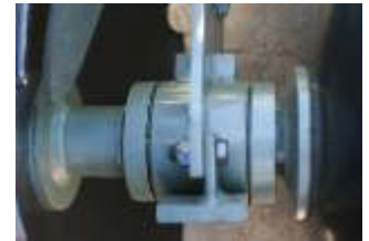
Erdvark maintenance free bearing unit.
