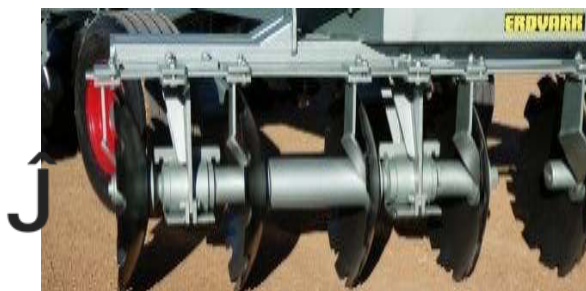
Erdvark maintenance free bearing unit.
